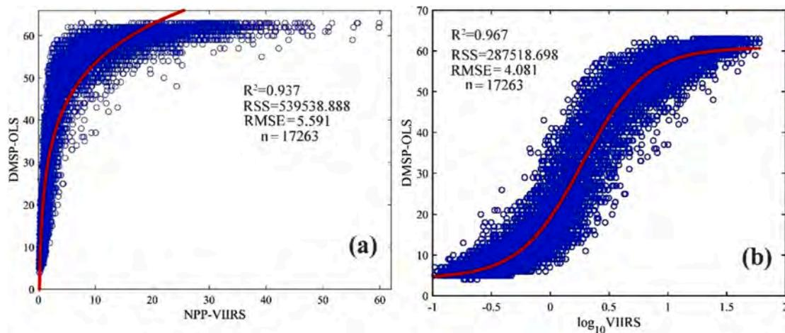
Fig. 2. Scatter plot of the original NPP-VIIRS and DMSP-OLS pixel pairs (a), and a scatter plot of logarithmically transformed NPP-VIIRS and original DMSP-OLS pixel pairs (b) in corresponding radiation-stable areas. The red curves denote the fitted model.
