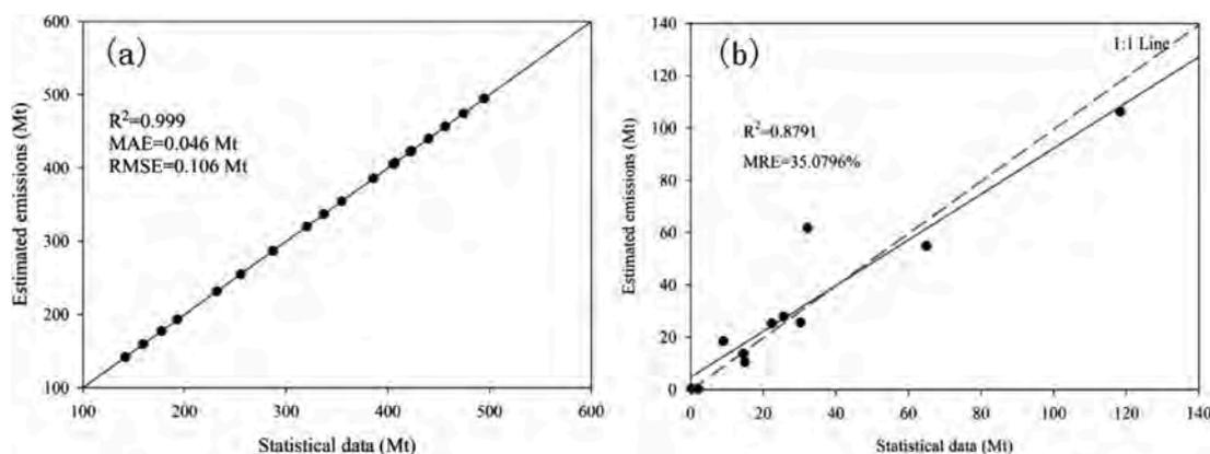
Fig. 6. Comparison of estimated CO<sub>2</sub> emissions and actual statistical CO<sub>2</sub> emissions. (a) Total fossil fuel related-energy CO<sub>2</sub> emissions of 2000-2018 in the GBA and (b) mean fossil fuel related-energy CO<sub>2</sub> emissions of 2000-2018 for 11 cities.
